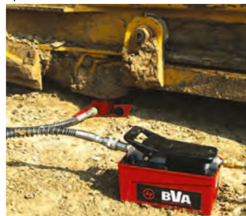
HF5006 in the collapsed position ready to lift a load with a PA1500 foot pump.
