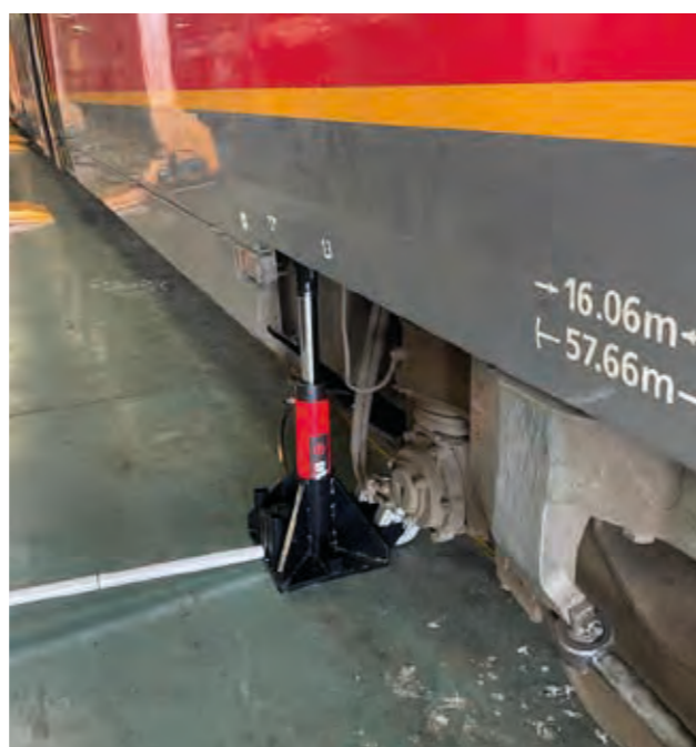
HD cylinders can be used in pushing and pulling applications. In this photo, we see a HD cylinder set up for a push application using a special designed mobile cylinder base plate.
