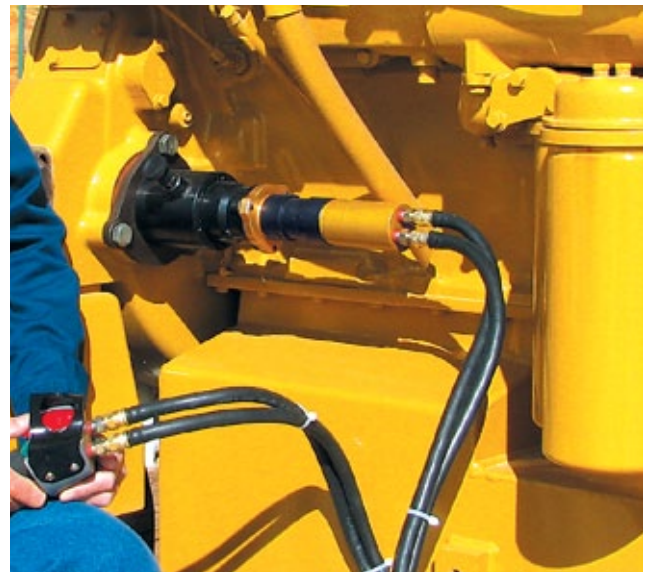
A B006PVR374-03-31P barring motor using pendant control, slow turning a Caterpillar 3408 engine.
