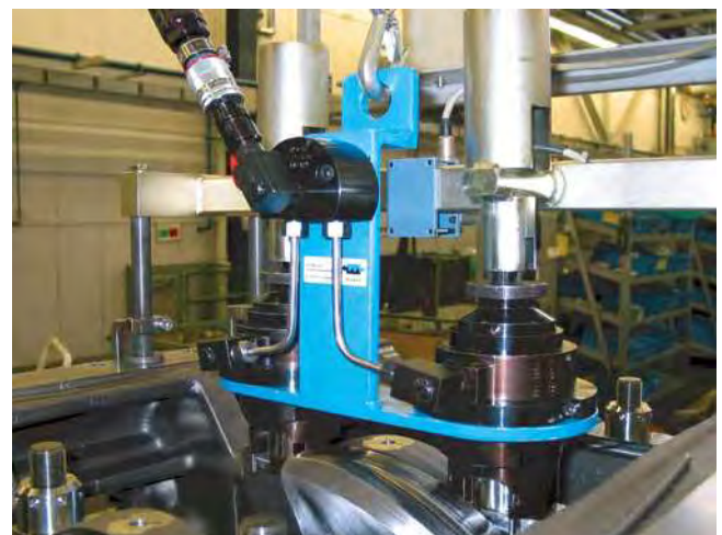
MDS in use on crankshaft bearing tensioners and as elongation controller - also optionally with pressure control.
